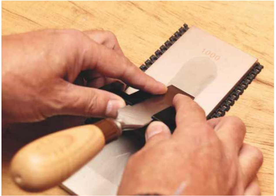
▲ The wide roller on the guide keeps things very stable as you work on the stone
